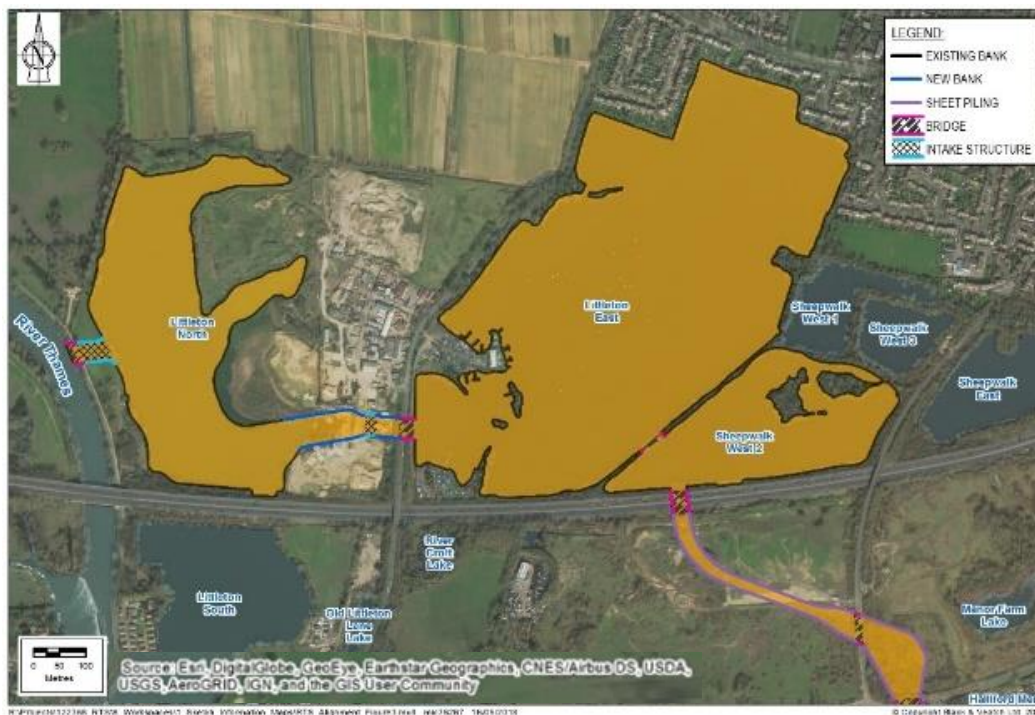
Channel extent following the removal of separation bund from Littleton East
