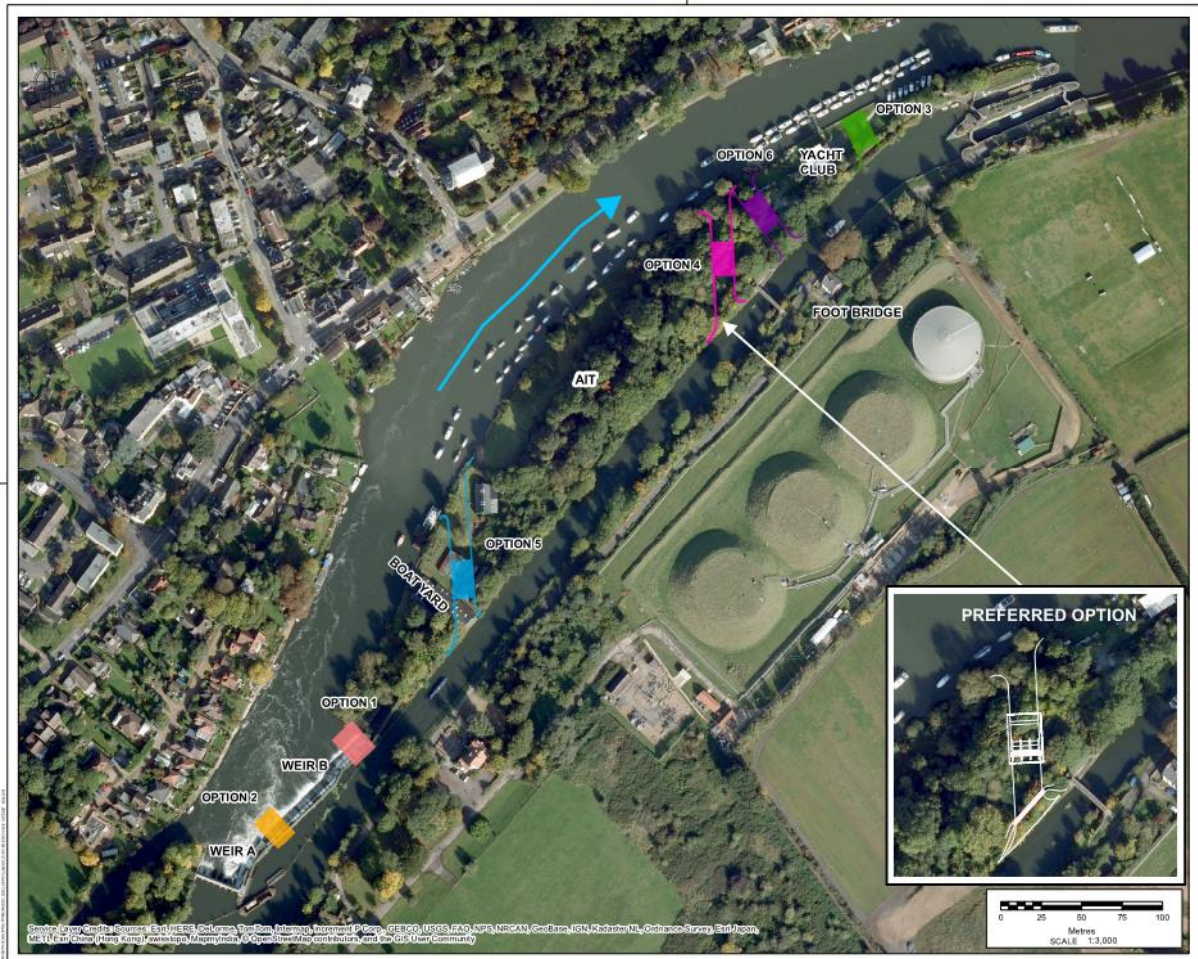
Alternative options considered for Sunbury weir capacity improvements (LTFRMS option = option 3; preferred option = option 4).
